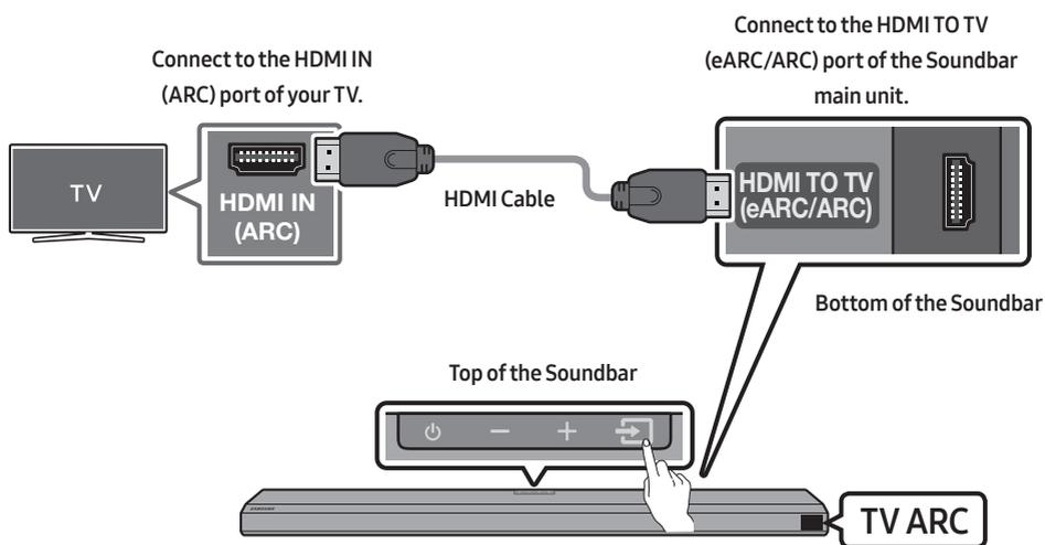
1. With the Soundbar and TV turned off, connect the HDMI cable as shown in the figure.
