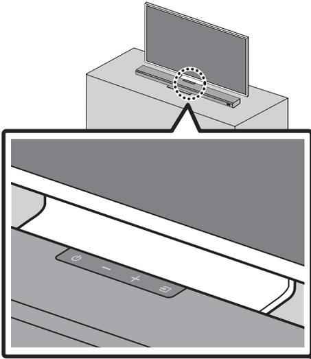
As illustrated in the image, align the center of the Soundbar with the center of the TV, carefully place the Soundbar onto the TV stand.
