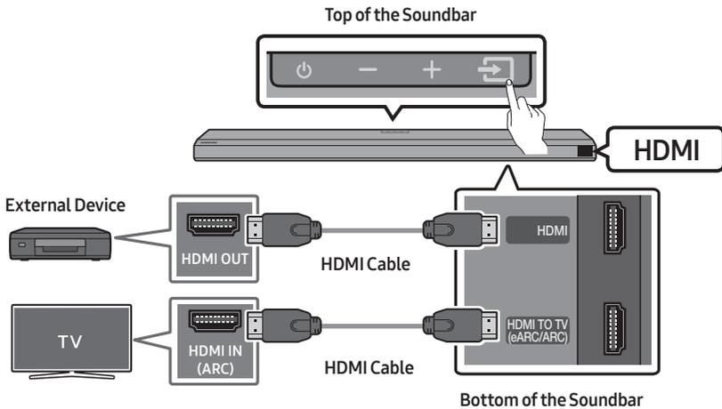
1. Use an HDMI cable to connect the HDMI OUT port on the external device and the **HDMI** port on the bottom of the Soundbar.
