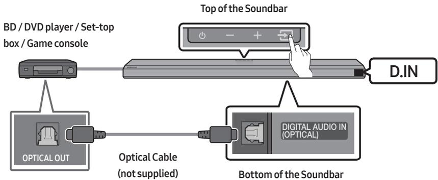
1. Use an optical cable (not supplied) to connect the **DIGITAL AUDIO IN (OPTICAL)** on the Soundbar main and the **OPTICAL OUT** port on the external device.
