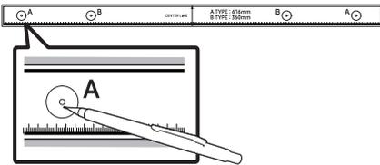
4. Using an appropriately sized drill bit, drill a hole in the wall at each marking.
