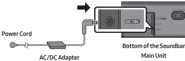
3. Connect power to the Soundbar and Subwoofer. The Subwoofer is automatically connected when the Soundbar is turned on.
