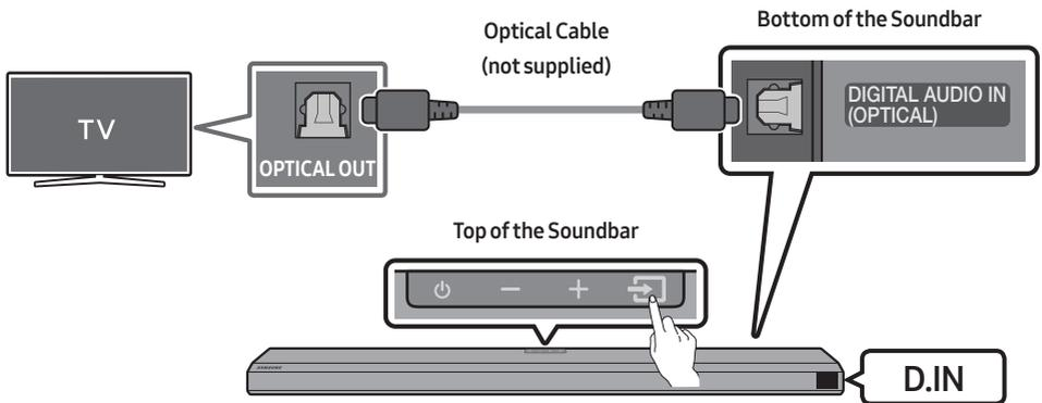
1. With the TV and Soundbar turned off, connect the **DIGITAL AUDIO IN (OPTICAL)** port on the Soundbar and the OPTICAL output port on the TV with the optical cable (not supplied), as shown in the figure.
