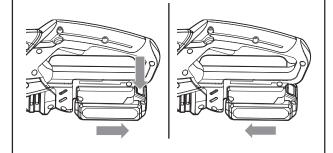
After recharging, insert the battery pack into the battery port. A simple push and slight pressure will be sufficient until a click is heard. Check to see if the battery is fully secured.
