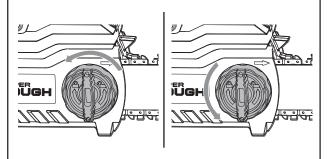
Grip the chain tensioning outer rim and turning it anti-clockwise to loosen the chain.
