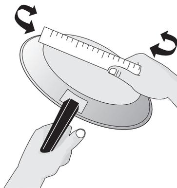
**Figure 2: Checking pan for flat bottom**
