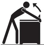
To check if the anti-tip bracket is installed properly, use both arms to grasp the rear edge of the appliance back. Carefully attempt to tilt
