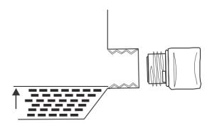
Figure 4: Engine Oil Correct Level
