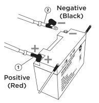
Figure 2: Installing Battery Leads
