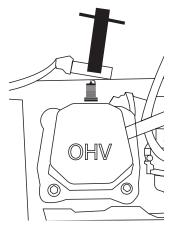
Figure 19: Remove Spark Plug
