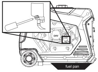
Figure 17: Loosen Float Bowl Screw
