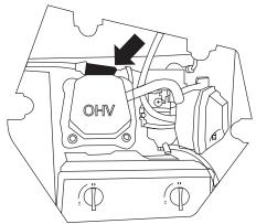
Figure 18: Pull off Spark Plug Cover
