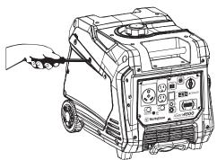
Figure 13: Remove Engine Service Panel
