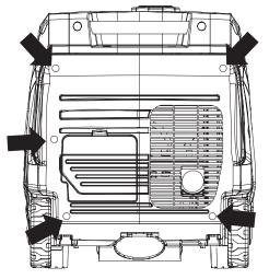
Figure 20: Remove Muffler Access Panel
