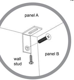
Secure L-bracket on the inside of panel A. See step 5 for detailed installation instructions.
