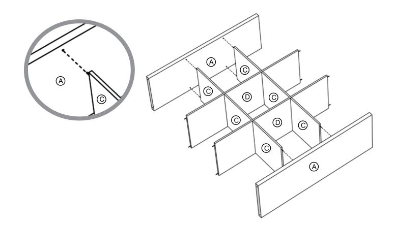
Align dowels on dividers (C) with center holes on both top/bottom panels (A).
