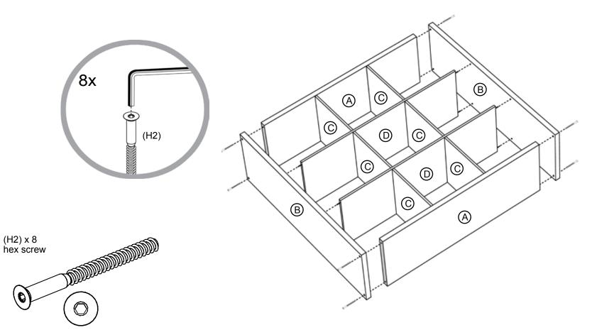
1. Align center holes in each side panel (B) with dowels in fixed shelves (D).
