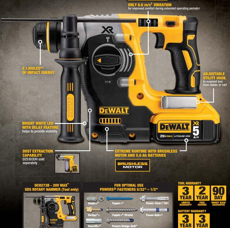
\*With respect to the 20V MAX: Maximum initial battery voltage (measured without a workload) is 20 volts. Nominal voltage is 18. \*\*According to EPTA-Procedure 05/2009. †Compared to hammers without vibration control. ICDCH273P2SS 9/15
