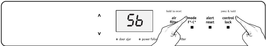
In the Sabbath mode, the High Temp alarm is active for health reasons. For example, if the door is left ajar the High Temp alarm is activated. The refrigerator will function normally once the door is closed without any violation of the Sabbath/holidays. The High Temp alarm is permitted when the cabinet temperature is outside the safe zone for 20 minutes. The alarm silences itself after 10 minutes while the High Temp icon stays lit until the Sabbath mode is exited.
