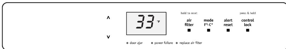
To adjust the temperature setting, press the UP (▲) key for warmer temperature and DOWN (▼) key for colder temperature on the control panel. Allow several hours for the temperature to stabilize between adjustments. The refrigerator can be adjusted between 33°F (1°C) and 46°F (8°C). By pressing the TEMP MODE key, the temperature display will toggle between °F and °C.
