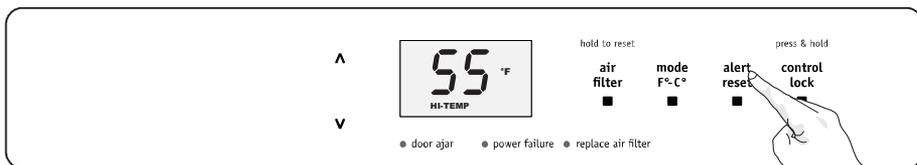
The audible alert can be turned off by pressing Alert RESET key.
