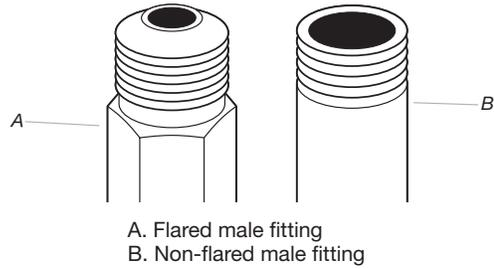
Remove red cap from gas pipe. Using a wrench to tighten, connect gas supply to dryer. Use pipe-joint compound on threads of all non-flared male fittings. If flexible metal tubing is used, be sure there are no kinks.
