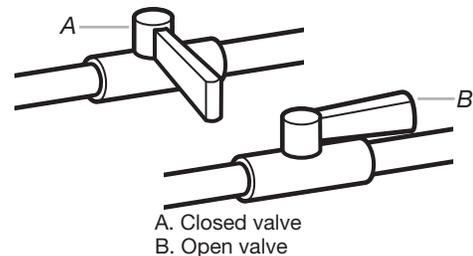
Open shut-off valve in supply line; valve is open when handle is parallel to gas pipe. Then, test all connections by brushing on an approved noncorrosive leak-detection solution. Bubbles will show a leak. Correct any leak found.
