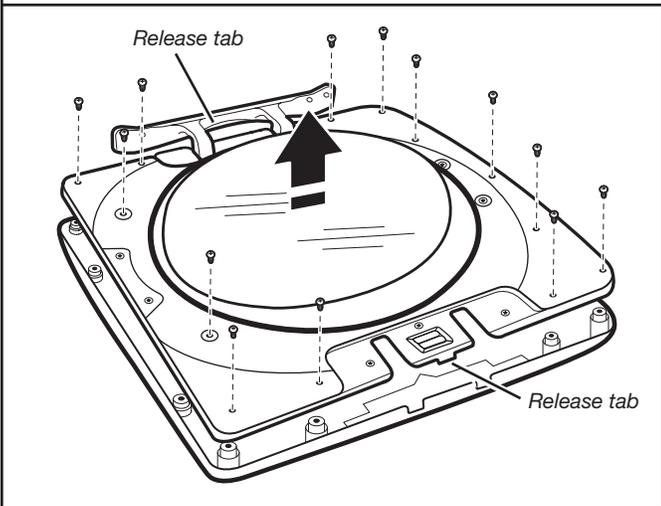
Position the door with the inside of the door facing up. Using a Phillips screwdriver, remove the 13 screws securing the inner door to the outer door. Lift off the inner door and set aside.
