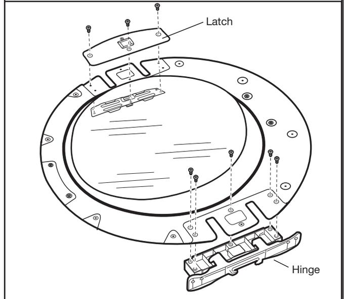
Using a TORX® T25® screwdriver, remove the three TORX® screws securing the latch plate and latch backing plate and the five screws holding the hinge assembly in place.
