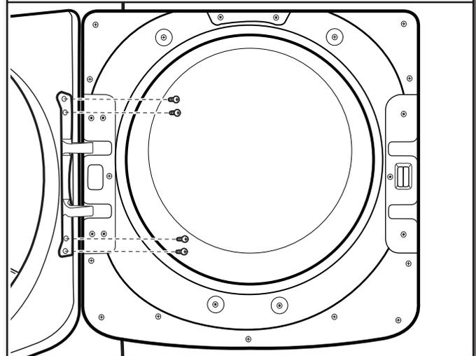
Using a TORX® T25® screwdriver, remove the four screws securing the door hinge to the dryer and lift up and out to remove the door. Place the door on a soft towel or other non-scratch surface. Retain or set aside the four screws.
