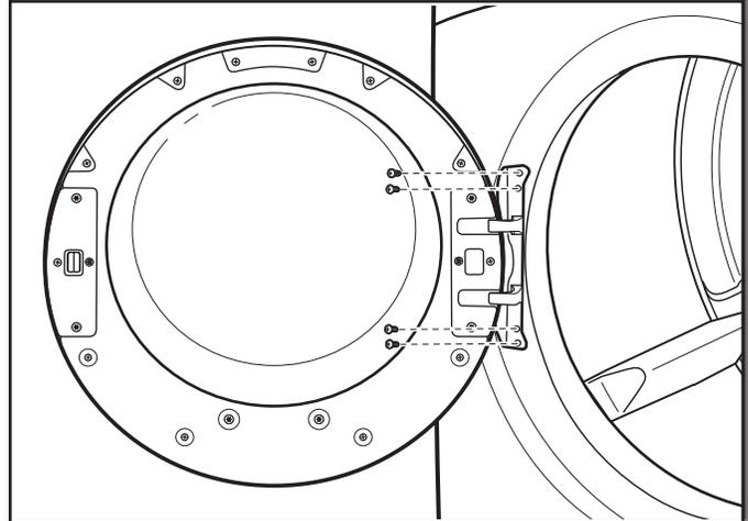
Using a TORX® T25® screwdriver, remove the four screws on the dryer. Insert the tabs on the hinge into the mounting slot and slide down to engage the top tab. Secure in place with the four TORX® T25® screws removed earlier.
