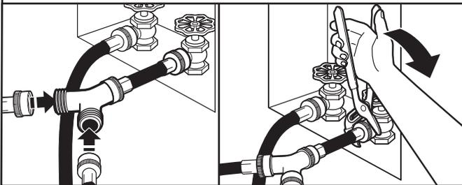
Attach one of the 5 ft. (1.5 m) inlet hose ends to the "Y" connector. Attach washer cold inlet hose to other side of "Y" connector. Screw on coupling by hand until it is seated on connector. Using pliers, tighten the couplings an additional 2/3 turn.
