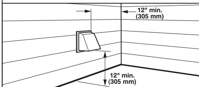
Install exhaust hood and use caulking compound to seal exterior wall opening around exhaust hood.
