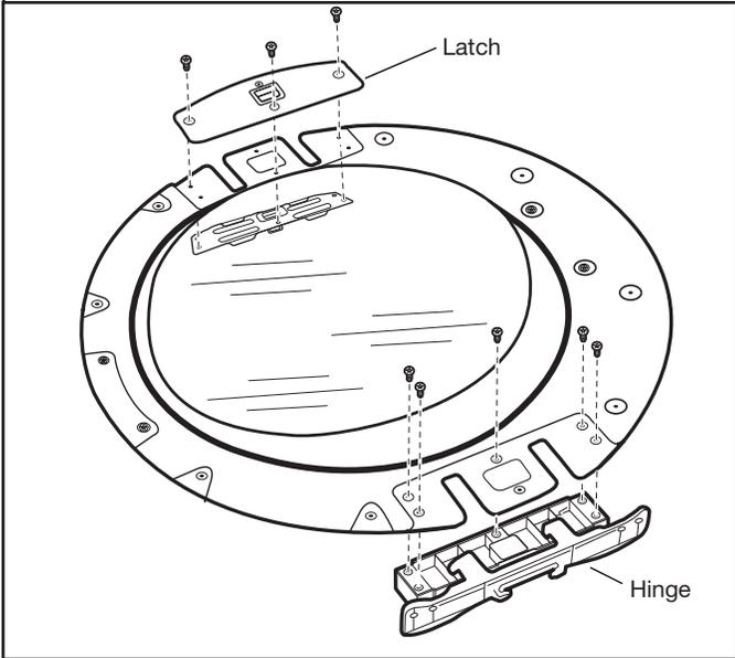
Using a TORX® T25® screwdriver, remove the three TORX® screws securing the latch plate and latch backing plate and the five screws holding the hinge assembly in place.
