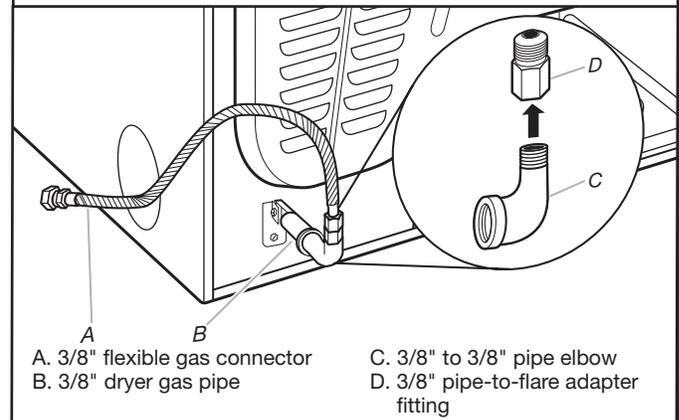
A combination of pipe fittings must be used to connect dryer to existing gas line. A recommended connection is shown. Your connection may be different, according to supply line type, size, and location.
