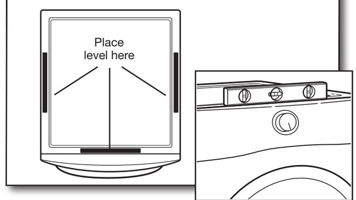
Check levelness of dryer from side to side. Repeat from front to back.
