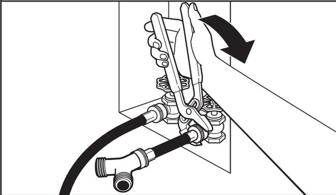
Using pliers, tighten the couplings with additional 2/3 turn.
