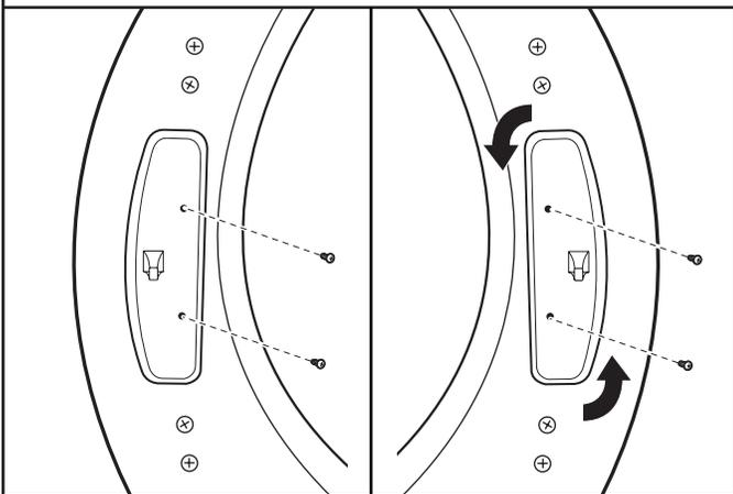
Using a TORX® T25® screwdriver, remove the two screws securing the door strike to the door frame of the dryer. Rotate the strike 180° and attach to the opposite side of dryer door frame, as shown.
