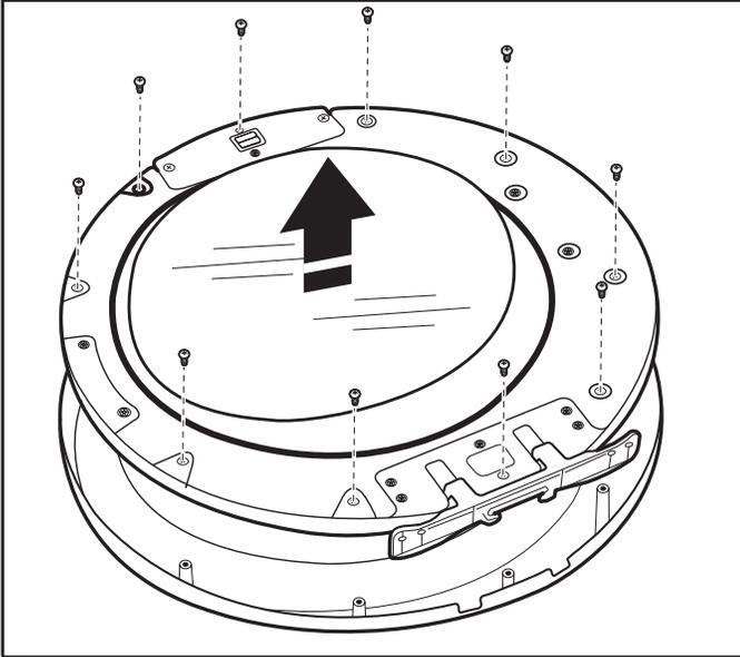
Position the door with the inside of the door facing up. Using a Phillips screwdriver, remove the 10 screws securing the inner door to the outer door. Lift off the inner door and set aside.
