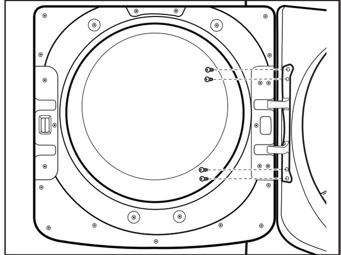
Using a TORX® T25® screwdriver, reinstall the four screws securing the door hinge to the dryer.
