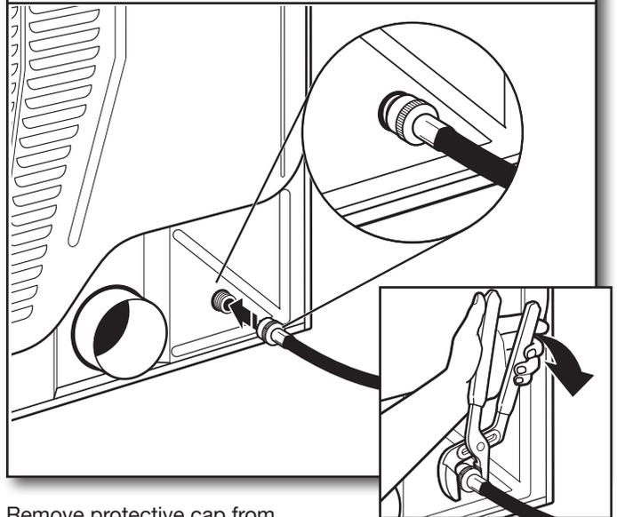
Remove protective cap from water inlet valve. Attach other end of long hose to fill valve at bottom of dryer back panel. Screw on coupling by hand until it is seated on fill valve connector. Using pliers, tighten the couplings an additional 2/3 turn.
