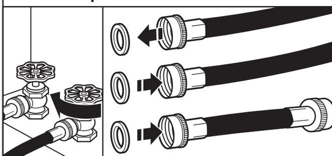
Turn cold water faucet off and remove washer inlet hose. Remove old rubber washer from inlet hose and replace with new rubber washer.
