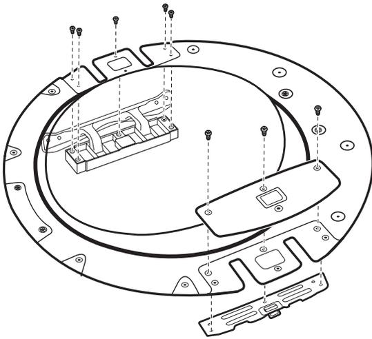
Using a TORX® T25® screwdriver, reinstall the latch plate and latch backing plate with the three TORX® screws removed earlier and the hinge assembly with the five screws on the opposite sides from which they were removed.
