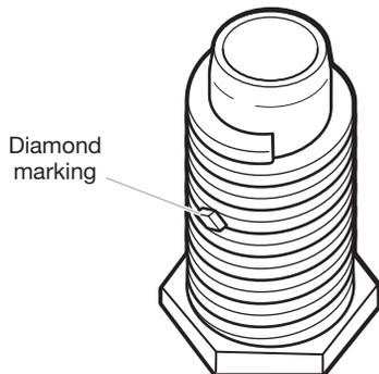
Examine leveling legs; find diamond marking. Screw legs into leg holes by hand, then use a wrench to finish turning legs until diamond marking is no longer visible.
