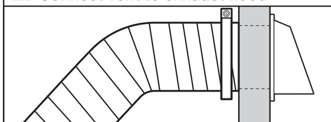
Vent must fit over the exhaust hood. Secure vent to exhaust hood with 4" (102 mm) clamp. Run vent to dryer location using straightest path possible. Avoid 90° turns. Use clamps to seal all joints. Do not use duct tape, screws, or other fastening devices that extend into interior of vent to secure vent because they can catch lint.
