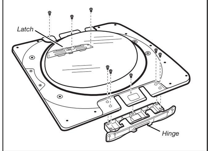
Using a TORX® T25® screwdriver, reinstall the latch plate and hinge assembly on the opposite sides from which they were removed.
