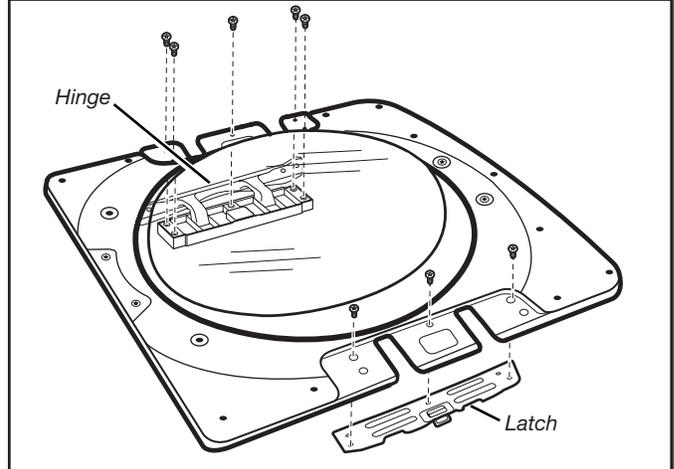
Using a TORX® T25® screwdriver, remove the three TORX® screws securing the latch plate and the five screws holding the hinge assembly in place.
