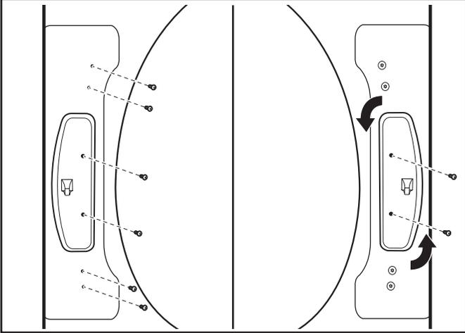
Using a TORX® T25® screwdriver, remove the two screws securing the door strike to the door frame of the dryer. Remove the four screws above and below the door strike and set aside for later use. Rotate the strike 180° and attach to the opposite side of dryer door frame, as shown.
