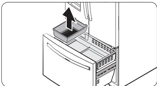
2. Lift the lower ice bucket to remove.
