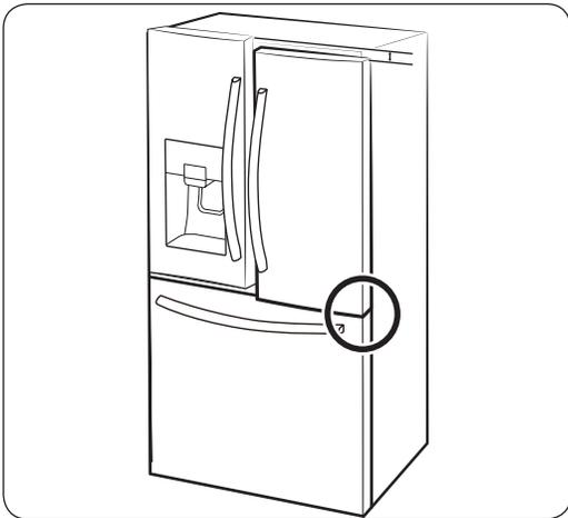
1. Check the height difference between the doors, and then lift up and hold the door with the lower height.
