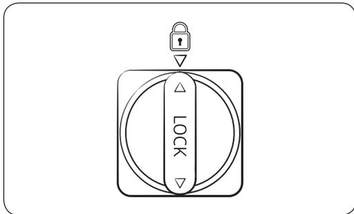
5. Turn the cartridge knob clockwise to lock into place.
