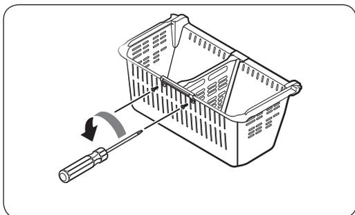
2. Use a Phillips screwdriver to unscrew the two screws affixing the **rear fixer** at the rear side of the basket.
