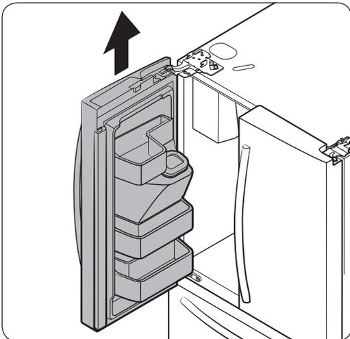
6. Gently pull up the door vertically to remove. Do not apply excessive force to the door. The door may fall, causing physical injury.
