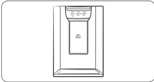
1. With the Ice Maker enabled, press **Cubed Ice** or **Crushed Ice** to select the ice type.
