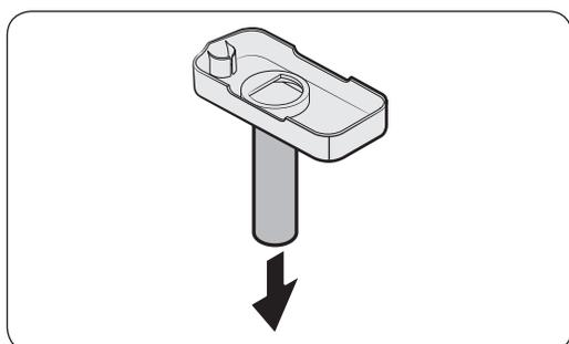
3. While slightly twisting the **infuser**, pull it out of the sealed mouth.
