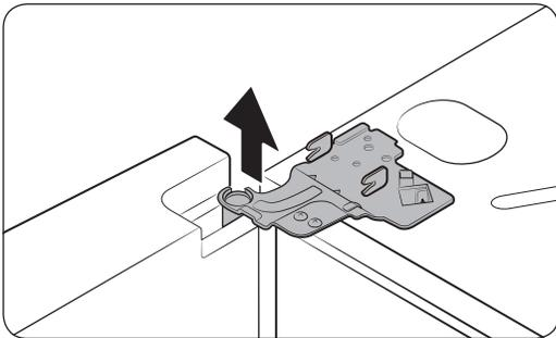
5. Open the door 90 degrees. While holding the door, pull up and remove the top hinge. Be careful not to damage the connector wires when you remove the hinge.
