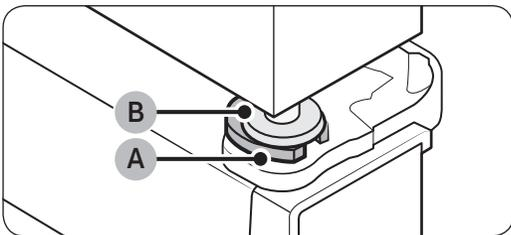
2. Insert a suitable-sized snap ring (A) between the door grommet (B) and the hinge as shown.
