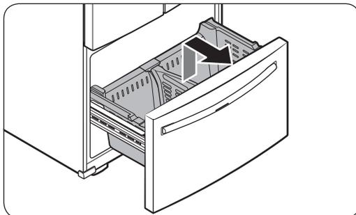
2. Then, pull up to remove the lower basket from the rail assembly.
