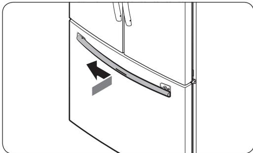
6. To attach the freezer handle to the refrigerator, first place the left side of the freezer handle onto the left handle screw, and then push it to the left.
