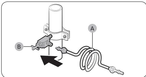
3. Connect the **water line installation kit (A)** to the **shutoff valve (B)**.
