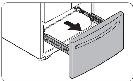
4. While holding the upper area of the freezer drawer front, slide the drawer out all the way to remove the freezer drawer from the rail assembly.
