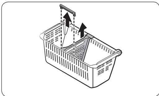
3. Pull the **rear fixer** and the **divider** upward to remove.
