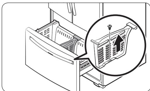
Loosen and remove the screw from the lower side of the divider. Then, pull straight up to remove the divider.
