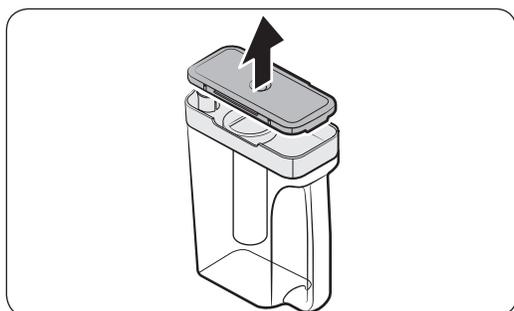
1. Grasp a handle groove of the **sealed mouth**, and then pull up to open the lid.
