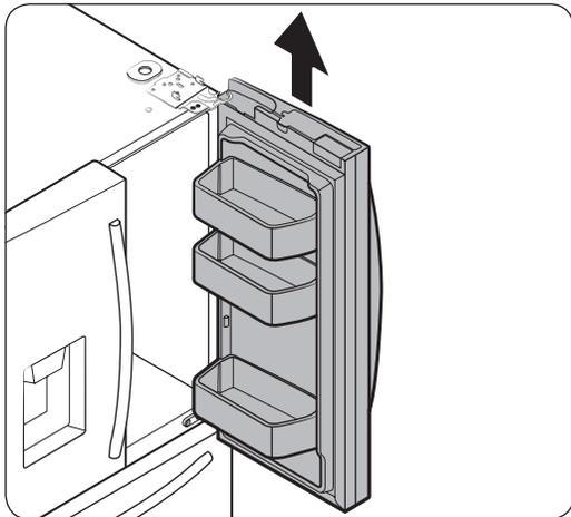
5. Gently pull up the door vertically to remove. Do not apply excessive force to the door. The door may fall, causing physical injury.
