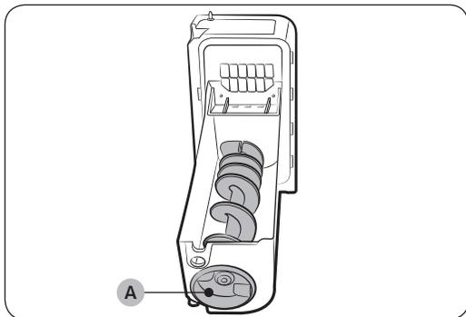
1. To remove the ice bucket, gently lift it up, and then pull it out slowly while holding the bottom of the bucket with one hand and the side with the other hand.
