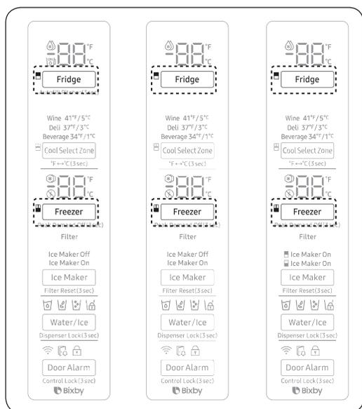
1. In this mode, the MAC address appears on the temperature panel (on both the freezer and the fridge sections of the panel) sequentially for 1 minute. Press and hold both **Freezer** and **Fridge** for 6 seconds. The temperature panel blinks. Then, press **Freezer** again to display the MAC address. The fridge beeps.
