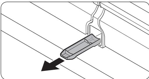
3. Pull out to remove the cartridge.
