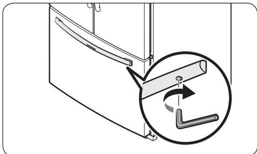
8. Insert the supplied wrench into the handle hole, and then turn it clockwise to tighten.
