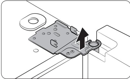
4. Open the door 90 degrees. While holding the door, pull up and remove the top hinge. Be careful not to damage the connector wires when you remove the hinge.
