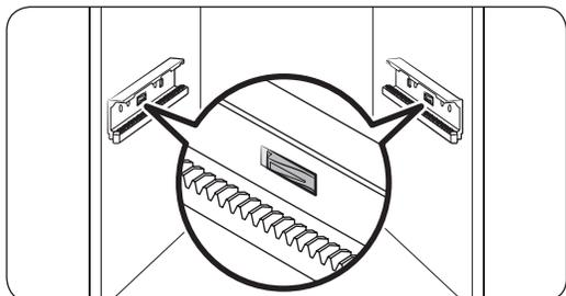
3. Press down the hooks to unlock the rail assembly.
