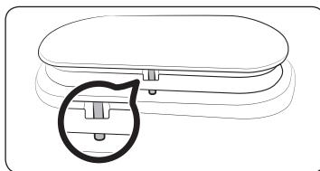
2. Install the burner head so that the electrode passes through the opening for the electrode. Make sure the burner head lies flat on the stove top.
