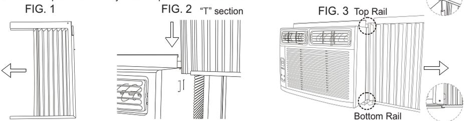
Your air conditioner is designed to install in standard double hung windows with opening widths of 23 to 36 inches (584 mm to 914 mm) (FIG. 4A , FIG. 4B).
