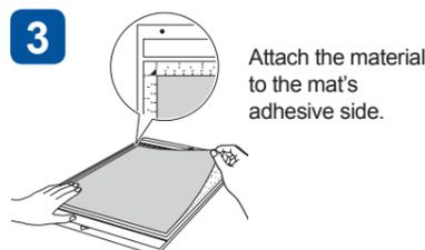
3 Attach the material to the mat's adhesive side.
