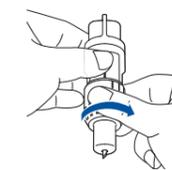
Fully turn the cap to the right to extend the blade tip to its maximum.
