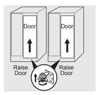
4. After leveling, verify door stop contacts lower hinge and top of door does not contact upper hinge through full movement of door (from fully closed to fully open).
