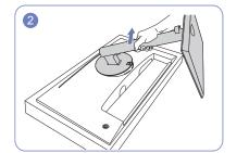
Place the product on a clean and flat floor as shown in Lift the stand neck in the arrow direction to detach it the figure. Push the key upward and hold. Turn the stand from the display. neck of the display counterclockwise for 10°.
