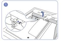
Place the product on a clean and flat floor as shown in Lift the stand neo the figure. Push the key upward and hold. Turn the stand from the display. neck of the display counterclockwise for 10°.
