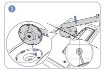
figure. When you place the stand neck, ensure that the raised button on the display can be inserted into the groove of the stand neck.
