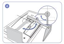
Place the stand neck on the display, as shown in the Turn the stand neck of the display clockwise for 90° to ensure that the stand neck of the display is put into place.
