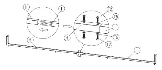
NOTE: The brackets' direction of the supporting bar H & I should keep the same. Do not tighten completely.
