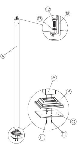
NOTE: The side with the counter sink hole should be outside for the bracket Q.
