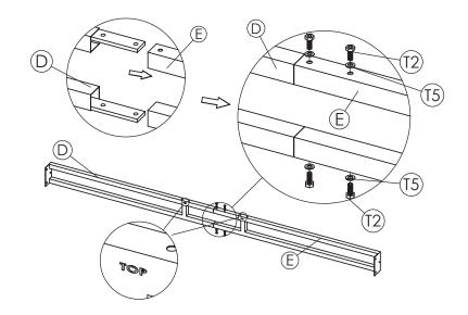
NOTE: The 'TOP' means the holes should be up. Do not tighten completely.
