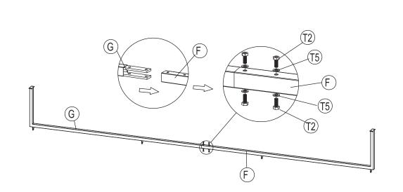
NOTE: The brackets' direction of the supporting bar F & G should keep the same. Do not tighten completely.
