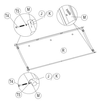
NOTE: The side marking the 'INSIDE' should face inside . Do not tighten completely.
