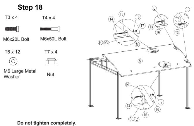
Repeat procedure for the other connection bar N and curved support bar L. Securely tighten all bolts and nuts.
