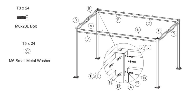
Do not tighten completely. Repeat procedure for the other three sides.
