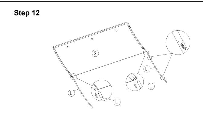
NOTE: The side marking the 'INSIDE' should face inside . Repeat procedure for the other curved support bar L.
