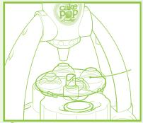
Insert tray with holes on top and align with nozzle. Be sure all tray clips are completely snapped in place.
