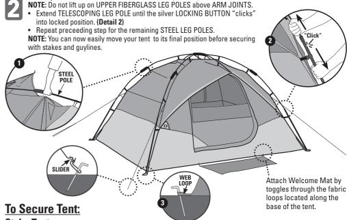
• Lift up on the STEEL POLE below ARM JOINT. (Detail 1)
